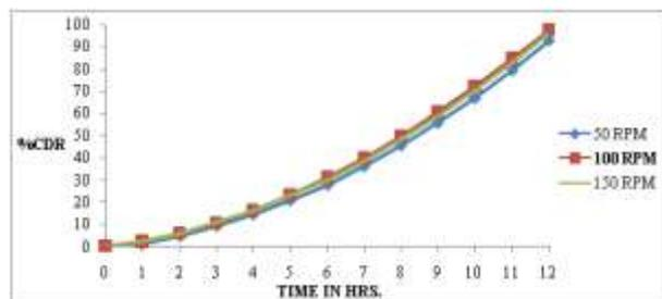
Fig. 6: It Shows Dissolution Profile Comparison through Change in Agitation Intensity of Media of FaC3.
