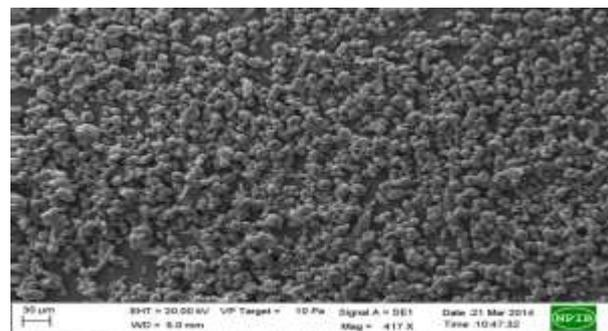
Fig. 7A: It Shows SEM Image of Membrane Containing PEG 6000 of Osmotic Tablet Before Dissolution Study of FaC3.
