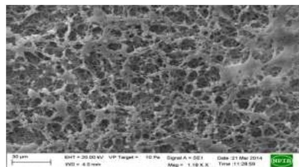
Fig. 7B: It Shows SEM Image of Membrane Containing PEG 6000 of Osmotic Tablet After Dissolution Study of FaC3.
