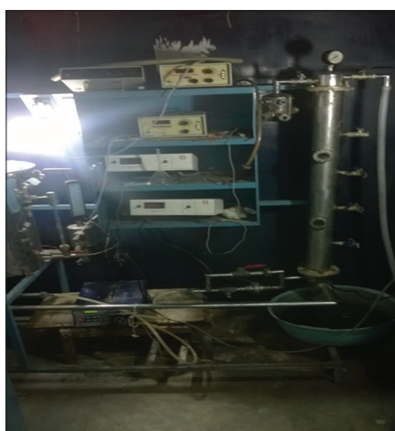
Fig. 1: Experimental setup with up-flow column reactor
