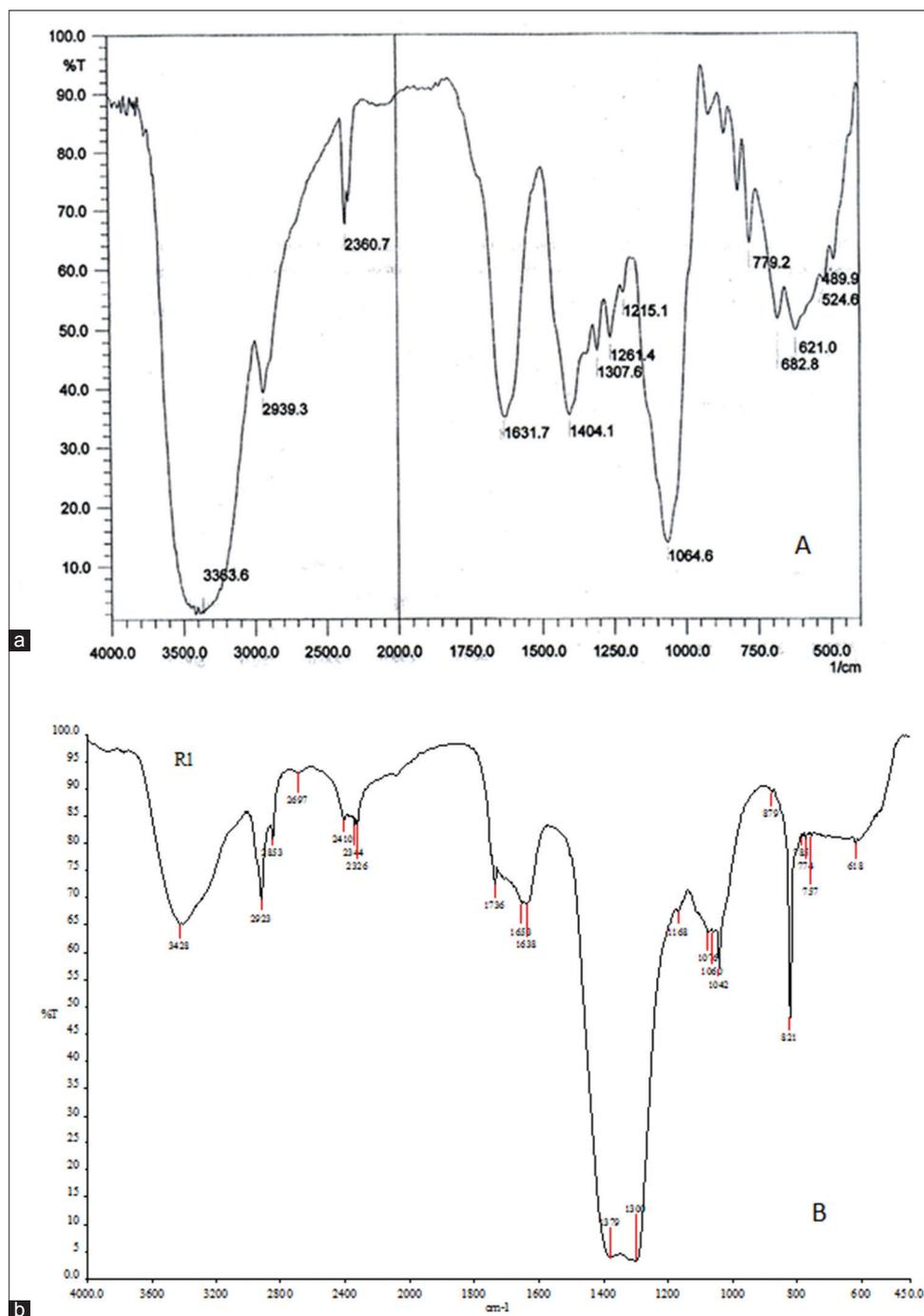
Fig. 2. Infrared-spectrum of taxol extracted sample from *Fusicoccum. Sp.* (a) Authentic taxol and, (b) extracted sample from *Fusicoccum. sp.*
