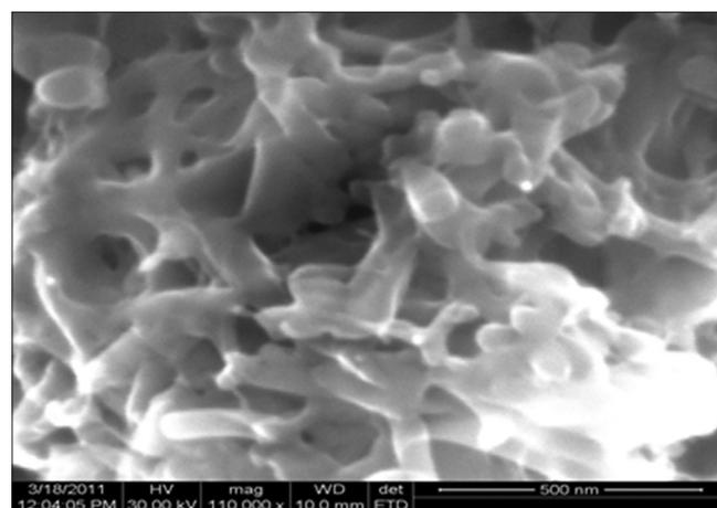
Fig. 1: Scanning electron microscopy photos of pramipexole dihydrochloride loaded methoxy polyethylene glycol-poly (caprolactone) nanosuspension (PMPNP 2)
