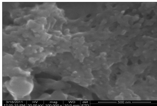
Fig. 2: Scanning electron microscopy photos of pramipexole dihydrochloride loaded methoxy polyethylene glycol-poly (caprolactone) nanosuspension (PMPNP 2)
