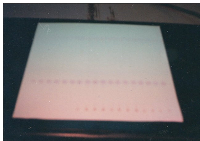
Fig. 1: Typical thin layer chromatography plates used (in this figure using the mobile phase chloroform: Acetone with paracetamol, simulation solution, Jamu A, Jamu B, and Jamu D)
