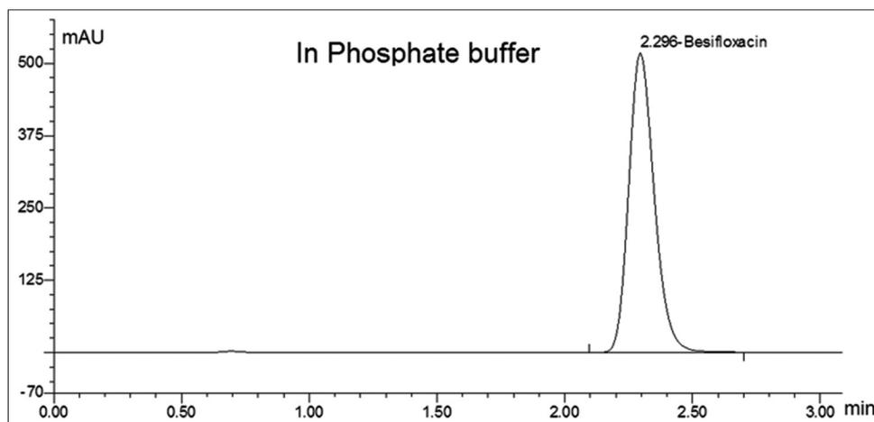
Fig. 4: Chromatogram of besifloxacin hydrochloride in phosphate buffer media
