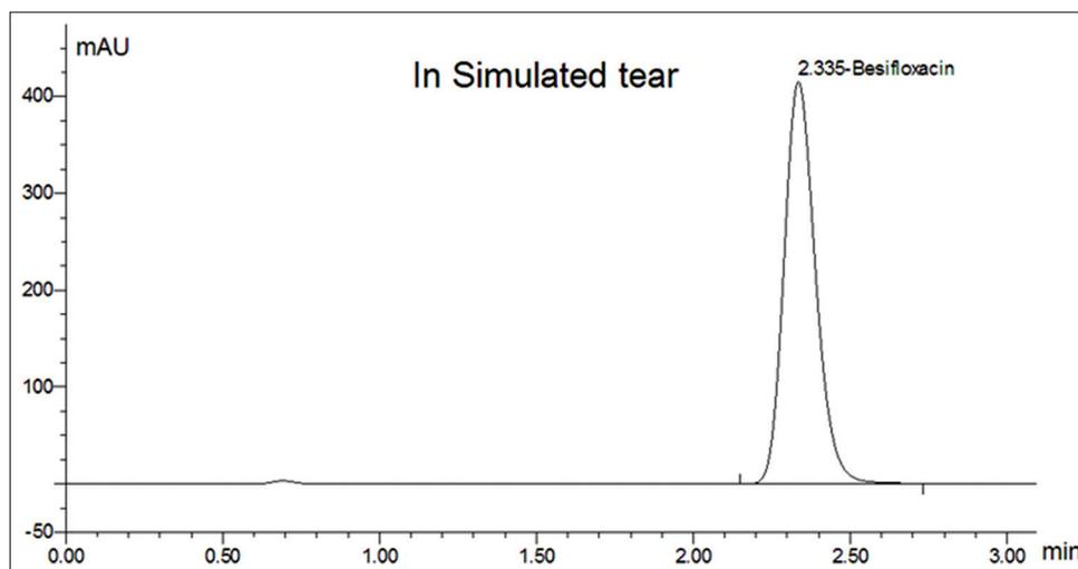
Fig. 5: Chromatogram of besifloxacin hydrochloride in simulated tear media
