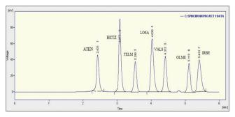
Fig. 1: A typical chromatogram showing the separation of atenolol and five angiotensin receptor blockade in the presence of hydrochlorothiazide mixture
