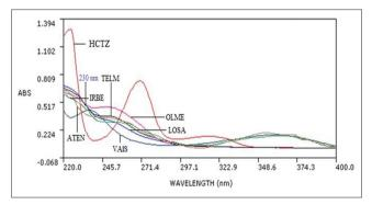
Fig. 2: Ultraviolet overlain spectra of the atenolol and five sartans with hydrochlorothiazide
