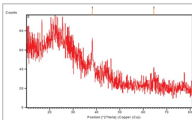
Fig. 5: X-ray diffraction spectra of silver nanoparticles from *Pleurotus florida*
