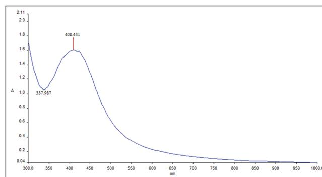
Fig. 1: Ultraviolet-visible spectrum of silver nanoparticle from *Pleurotus florida*
