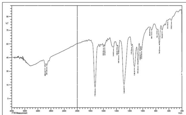
Fig. 2: Fourier transmission infrared spectrum of silver nanoparticle from *Pleurotus florida*
