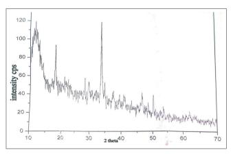
Fig. 3: X-ray diffraction pattern of chitosan
