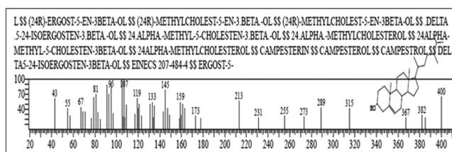
Fig. 4: Mass spectrum of ergost-5-en-3-ol, (3.beta., 24r)-
