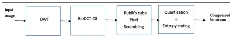
Fig. 2: Proposed system architecture
