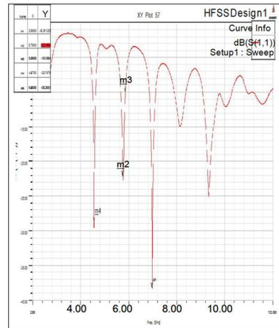
Fig. 4: S (1,1) of the first antenna
