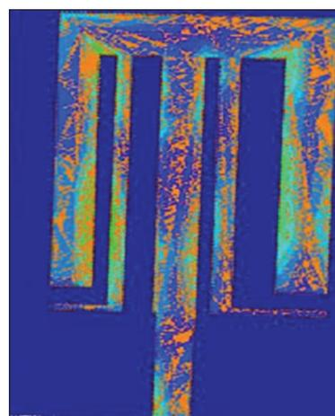
Fig. 8: Current density distribution of the first antenna design at 3.4 GHz
