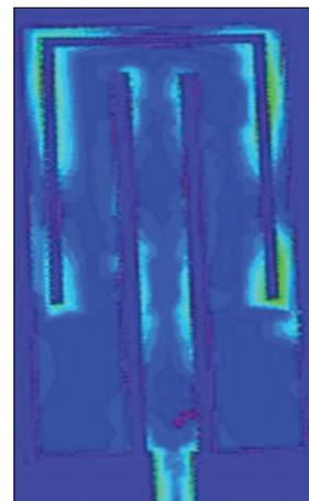
Fig. 7: Current density distribution of the first antenna design at 5.8 GHz
