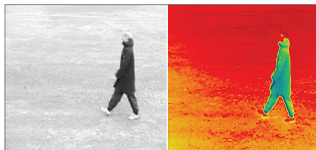
Fig. 1: Sample result of the compressed depth map created by the proposed algorithm from the given input video sequence and facilitating sharing the mapped data over a network
