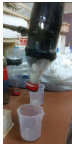
Fig. 4: Activated charcoal layer and cotton layer compartment
