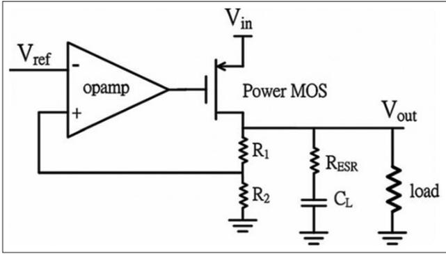
Fig. 1: Basic low dropout schematic
