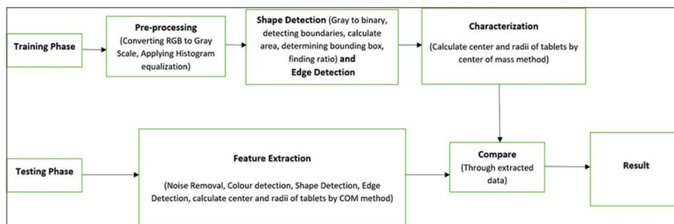
Fig. 1: Architectural diagram for characterization of pharmaceutical blisters
