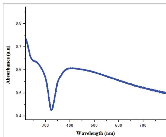
Fig. 3: Ultraviolet-visible spectra of silver nanoparticles synthesized by *Aspergillus* extract of *Withania somnifera*
