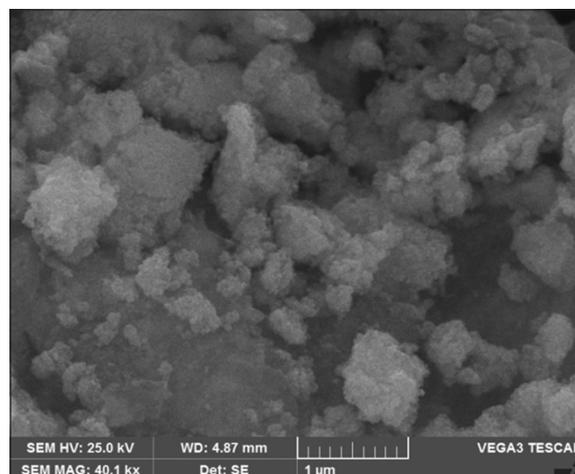
**Fig. 5: Scanning electron microscopy images of silver nanoparticle**
