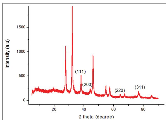
**Fig. 4: X-ray diffraction pattern of silver nanoparticles**
