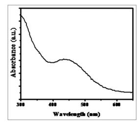
Fig. 1: Ultraviolet-visible spectrum of silver nanoparticles
