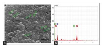
Fig. 2: (a) Scanning electron microscope micrograph of approach to synthesize silver nanoparticles and (b) corresponding energy dispersive X-ray spectrum
