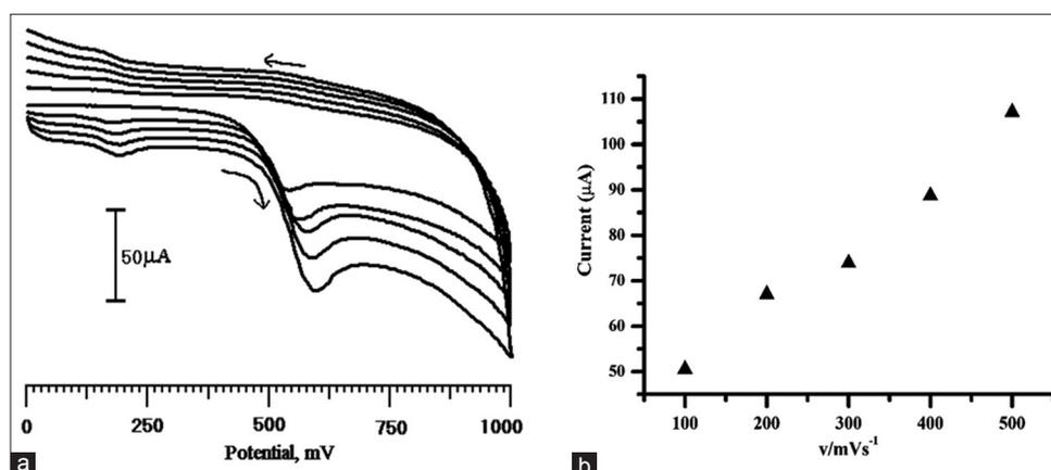
Fig. 6: (a) Cyclic voltammograms of 1 mM resorcinol (RS) at the SDSMCNTGMPE in pH 7 phosphate buffer solutions at various scan rates. From: 100, 200, 300, 400, and 500 mV/s. (b) Plot of the peak current of RS as a function of the scan rate
