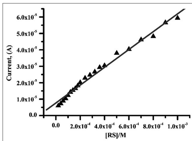
Fig. 8: Calibration plot for the determination of resorcinol at the SDSMCNTGMPE in pH 7 phosphate buffer solutions with the scan rate 100 mV/s
