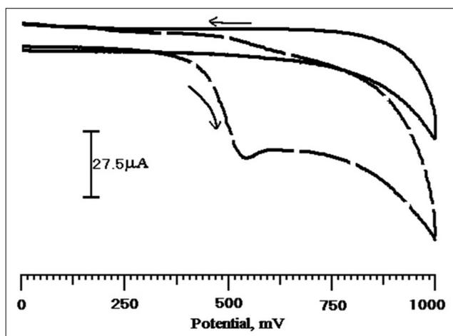
Fig. 3: A typical cyclic voltammograms of SDSMCNTGMPE with 1 mM resorcinol (RS) in pH 7. Phosphate buffer solutions (PBSs) (dashed line) without 1 mM RS at pH 7. PBS blank (solid line)
