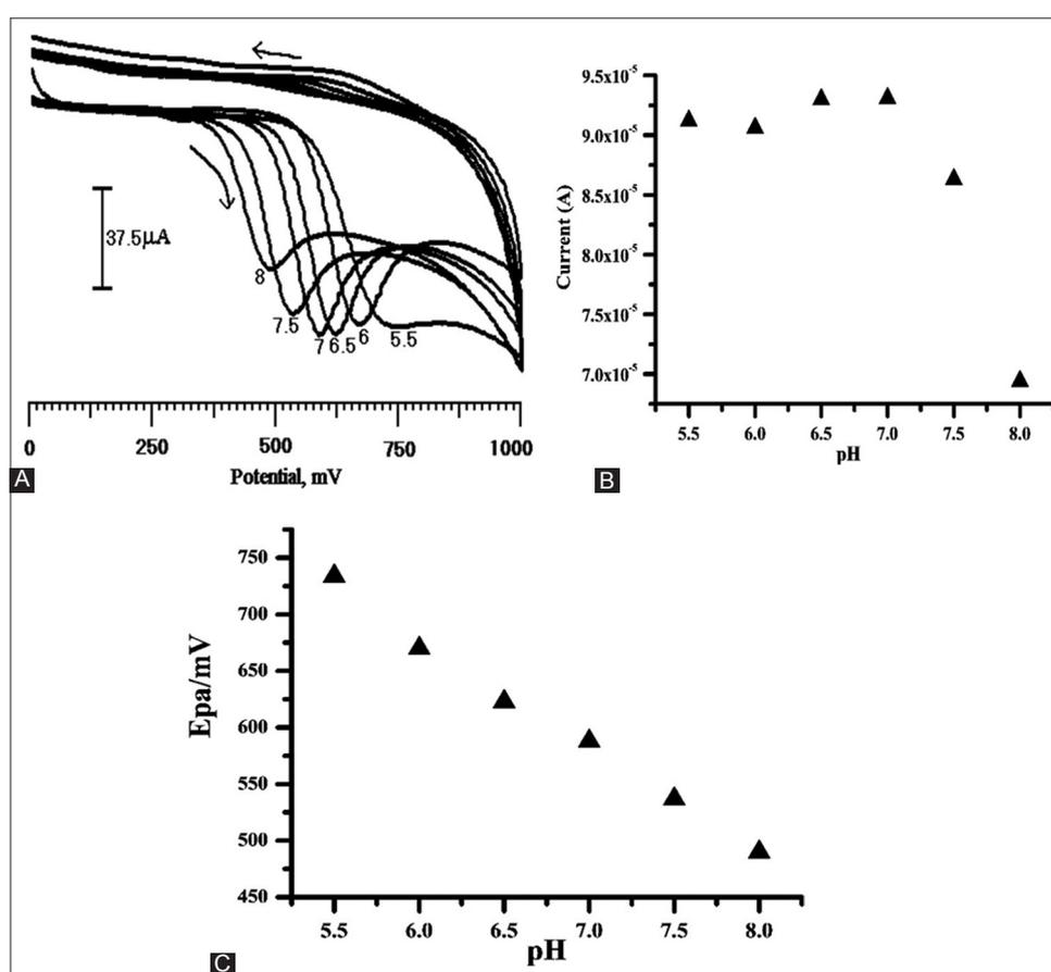
Fig. 7: (A) Cyclic voltammograms obtained at the SDSMCNTGMPE in 0.2 M phosphate buffer solutions in pH values, (a) 5.5 (b) 6 (c) 6.5 (d) 7 (e) 7.5 (f) 8 containing 1 mM resorcinol (RS), (B) plot of anodic peak current versus pH (5.5-8.0) of 1 mM RS at the SDSMCNTGMPE, (C) plot of Epa versus pH for RS
