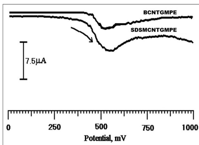
Fig. 5: DPVs of a solution containing 1 mM resorcinol in 0.2 M phosphate buffer solutions (pH 7) at the BCNTGMPE and SDSMCNTGMPE
