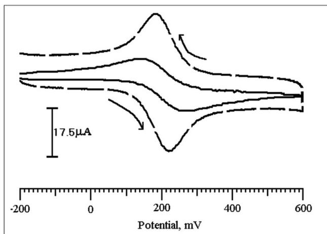
Fig. 2: Cyclic voltammograms of 1 mM potassium ferrocyanide at the BCNTGMPE (solid line) and at the SDSMCNTGMPE (dashed line) in 1 M KCl
