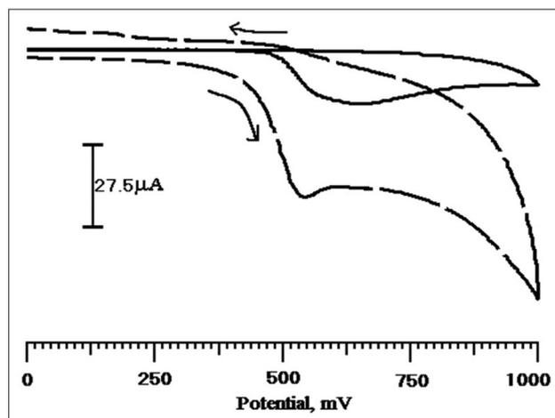
Fig. 4: Cyclic voltammograms of 1 mM resorcinol in pH 7 phosphate buffer solutions at the BCNTGMPE (solid line), the SDSMCNTGMPE (dashed line)
