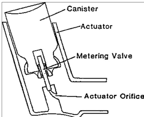
Fig 1: Schematic diagram of a metered-dose inhaler [14]
