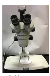
Fig. 5: Stereomicroscope
