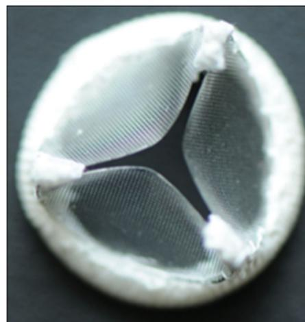
**Fig. 1: Hybrid valve from polymer**
