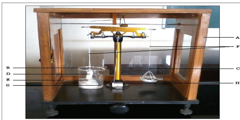
Fig. 3: *In vitro* bioadhesive strength measurement. (a) *In vitro* bioadhesive strength measurement modified balance apparatus, (b) left pan, (c) right pan, (d) teflon cylinder, (e) goat mucosa, (f) threads, (g) beaker containing solution, (h) pointer
