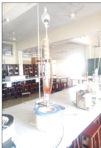
Fig. 1: Soxhlet apparatus used to prepare an aqueous extract of tobacco from cigarette
