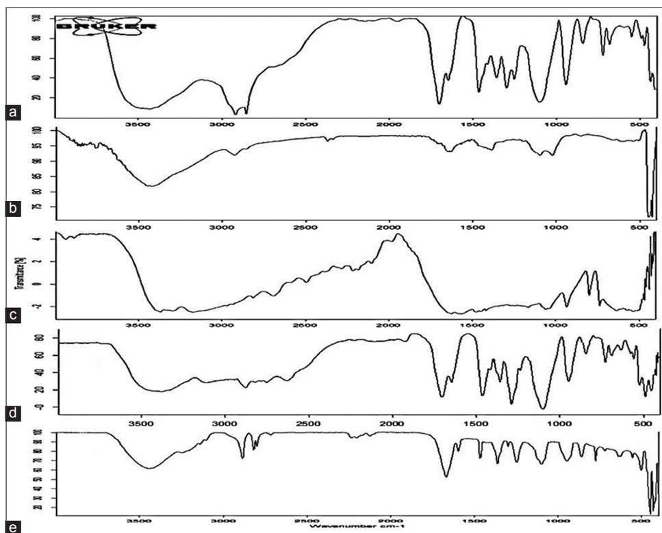
Fig. 2: Fourier transform infrared spectra of (a) SAF127 copolymer, (b) polyvinyl alcohol, (c) metformin, (d) physical mixture, and (e) MN3
