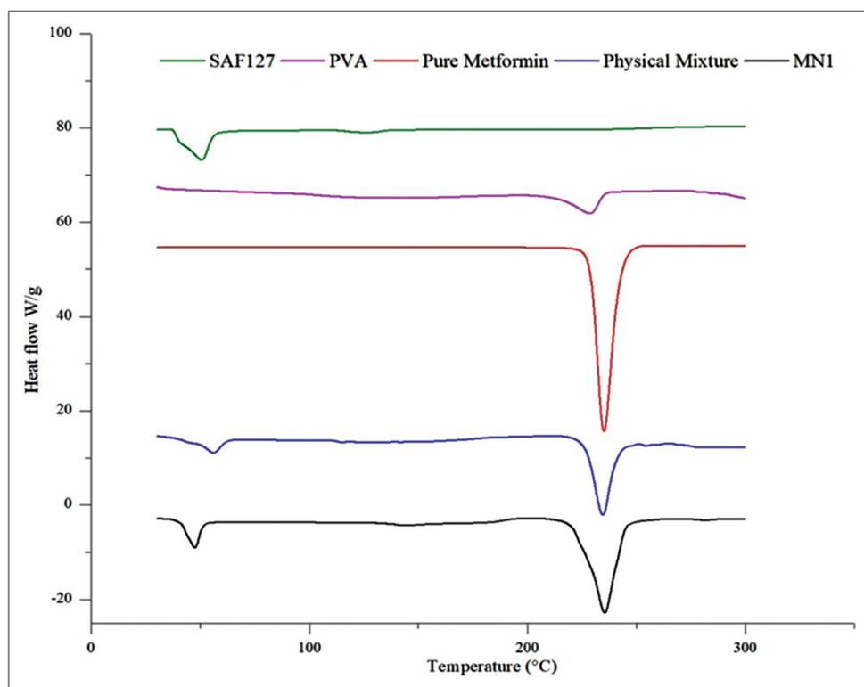
Fig. 3: Differential scanning calorimetry thermogram of SAF127 copolymer, polyvinyl alcohol, pure metformin, physical mixture, and MN3
