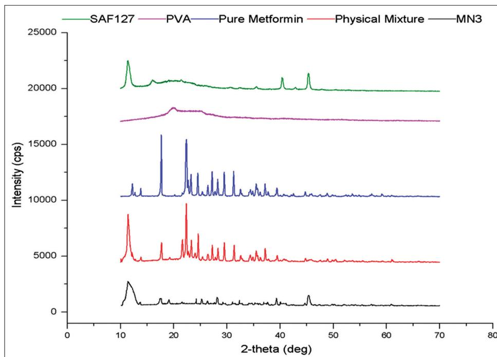
Fig. 4: X-ray diffractometer patterns of SAF127, polyvinyl alcohol, pure metformin, physical mixture, and MN3
