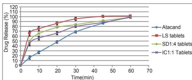
**Fig. 10: Dissolution profile of candesartan cilexetil from the prepared tablets and the marketed product**
