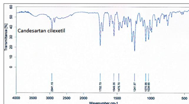
**Fig. 1: Fourier transform infrared spectrum of candesartan cilexetil**
