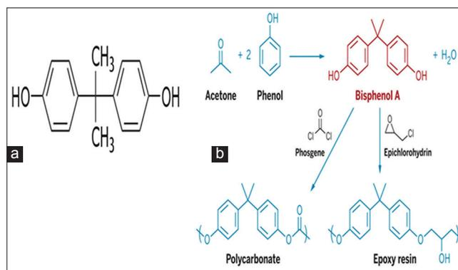
Fig. 1: (a) Chemical structure of bisphenol A (BPA), (b) Chemical transformation from BPA to polycarbonate and epoxy resin
