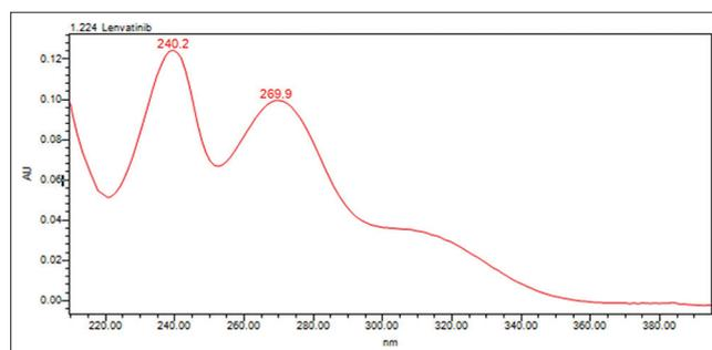
Fig. 2: Ultraviolet spectrum of lenvatinib
