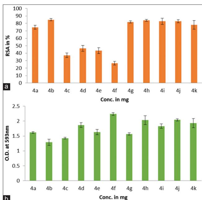
Fig 1: Radical scavenging activity (RSA) of pyrano[2,3-d]pyrimidinediones (a) 1,1-diphenyl-2-picrylhydrazyl RSA in (b) ferric reducing antioxidant power expressed in O. D. at 593 nm
