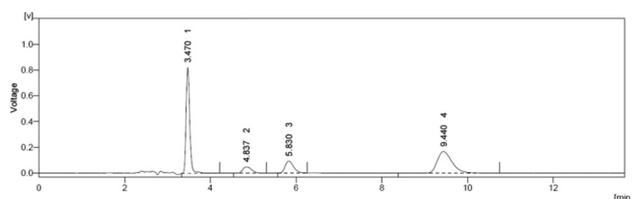
**Fig. 3: Chromatogram of metformin (1), sitagliptin (2), pioglitazone (3), and glimepiride (4) in 20 mM potassium dihydrogen phosphate buffer (pH 4.0): acetonitrile (65:35 %v/v) with flow rate - 1.0 ml/min**
