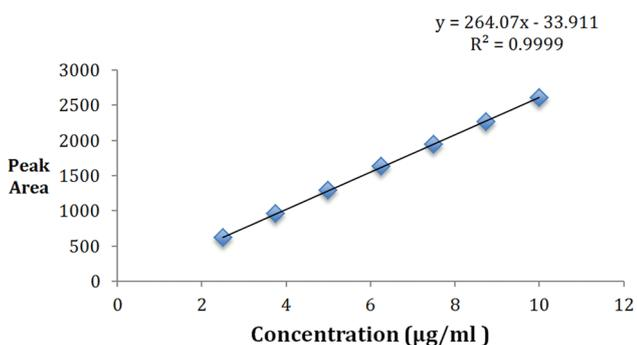
Fig. 5: Standard calibration curve of sitagliptin (2–10 µg/ml)
