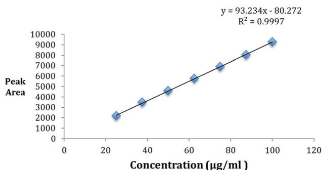
Fig. 4: Standard calibration curve of metformin (25–100 µg/ml)
