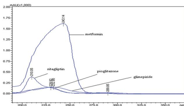
**Fig. 2: Overlay ultraviolet spectrum of metformin, sitagliptin, pioglitazone, and glimepiride showing selection of wavelength detection**
