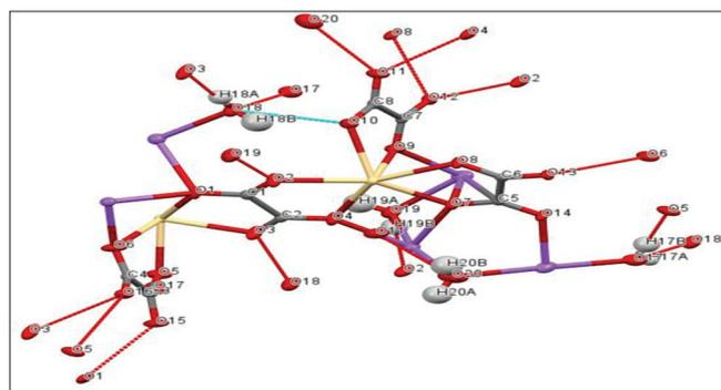
Fig. 2: The intermolecular hydrogen bonds metal-oxygen bonds of the sodium cadmium oxalate structure
