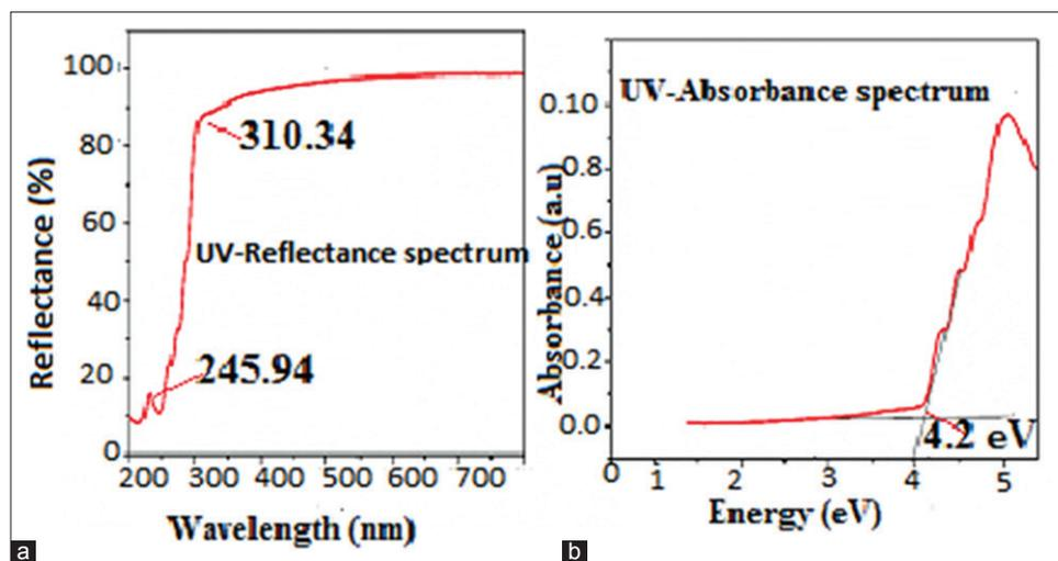
Fig. 3: Diffused reflectance spectrum of (a) sodium cadmium oxalate; absorbance spectrum of (b) sodium cadmium oxalate
