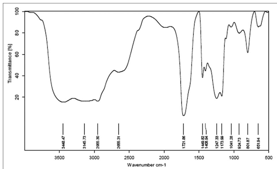
Fig. 2: Fourier-transform infrared spectrum of Carbopol 940
