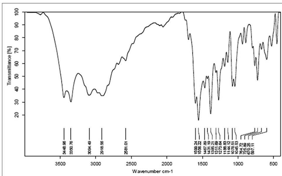
Fig. 1: Fourier-transform infrared spectrum of itraconazole
