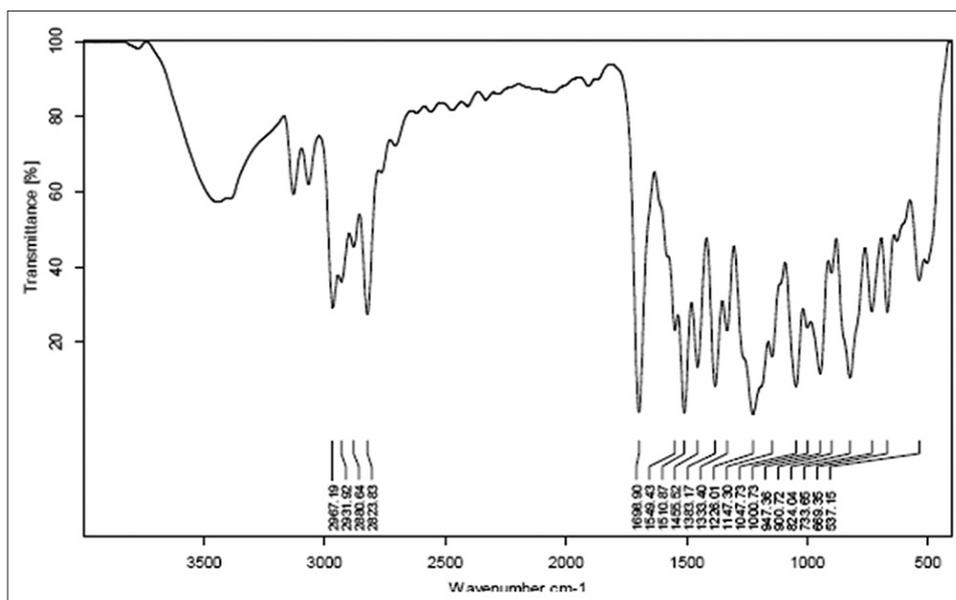
Fig. 3: Fourier-transform infrared spectrum of drug + polymer
