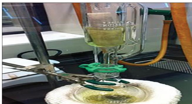
Fig. 3: Soxhlet extractor of plant
