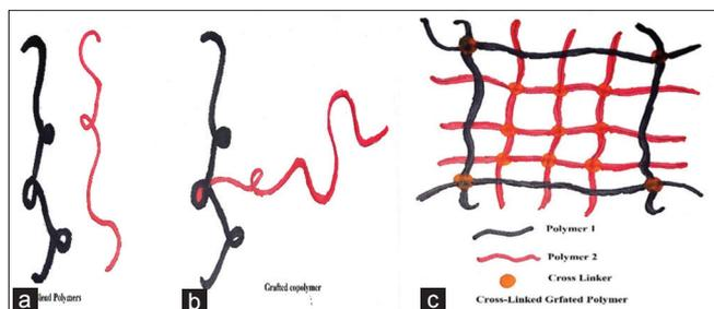
Fig. 1: (a) Blend polymer, (b) grafted polymer and (c) cross-linked grafted polymer
