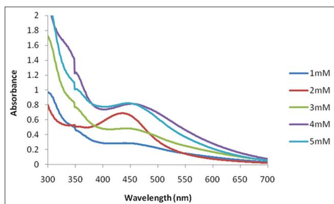
Fig. 4: Ultraviolet-visible spectrum of the silver nanoparticles synthesized at different concentration of silver nitrate
