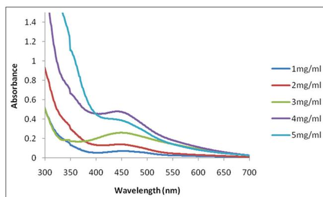
Fig. 1: Ultraviolet-visible spectrum of the silver nanoparticles synthesized using a different concentration of plant extract
