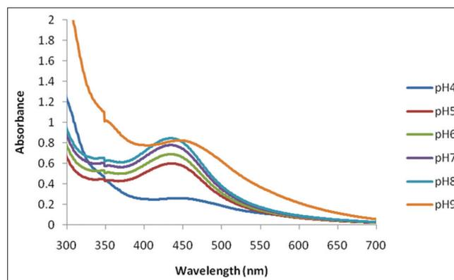
Fig. 3: Ultraviolet-visible spectrum of the silver nanoparticles synthesized at different pH
