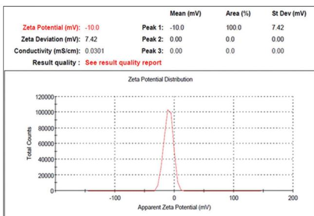
Fig. 8: Zeta potential analysis of synthesized silver nanoparticles
