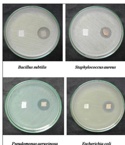
**Fig. 9: Antibacterial activity of the cotton fabric incorporated with silver nanoparticles**
