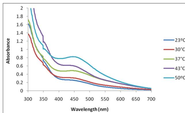
Fig. 2: Ultraviolet-visible spectrum of the silver nanoparticles synthesized at the different reaction temperature
