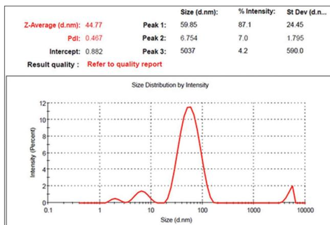
Fig. 7: Dynamic light scattering analysis of synthesized silver nanoparticles
