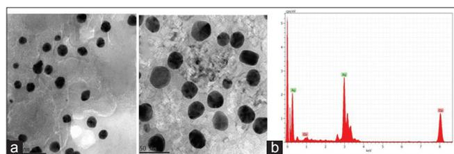
Fig. 6: (a) Transmission electron microscopy and (b) energy dispersive X-ray analysis of synthesized silver nanoparticles
