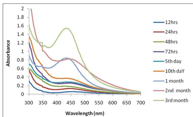
Fig. 5: Ultraviolet-visible spectrum of the silver nanoparticles at different time durations
