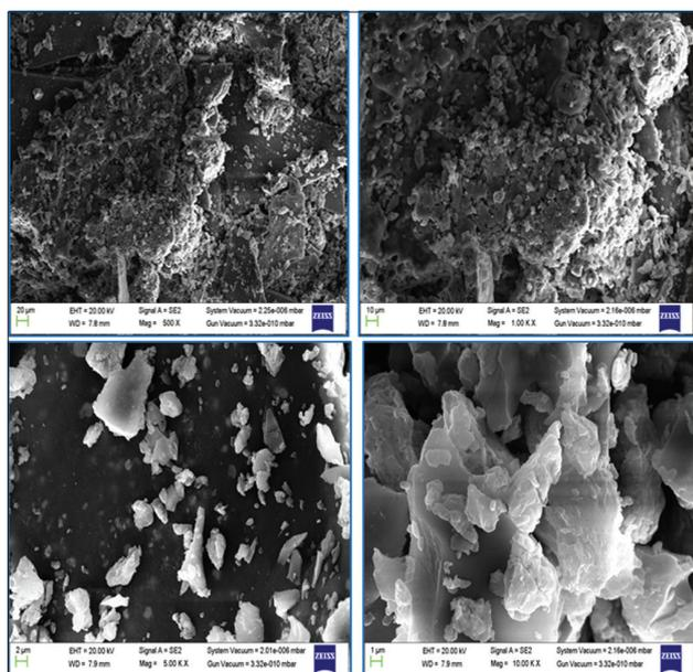
Fig. 3: Field emission scanning electron microscopy (FESEM) images of silver nanoparticles (AgNPs) synthesized using extract of *Ipomoea batatas*
