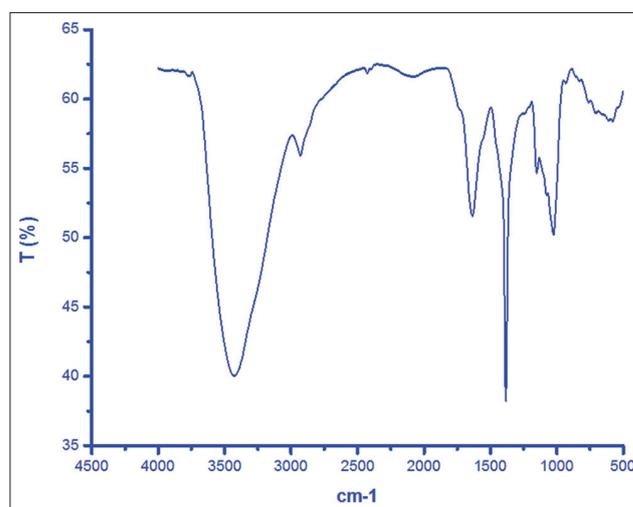
Fig. 1: Fourier-transform infrared spectroscopy spectra of silver nanoparticles synthesized using extract of *Ipomoea batatas*
