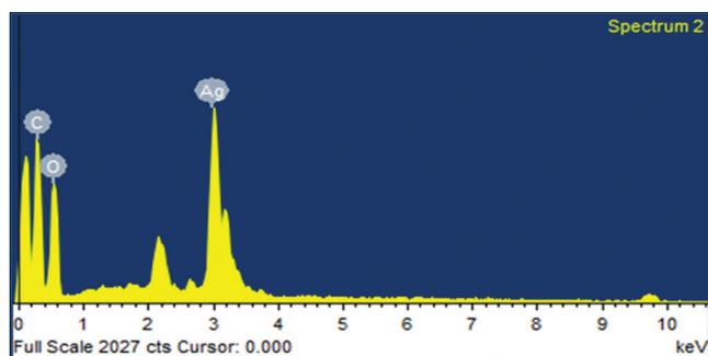
Fig. 4: Energy dispersive X-ray spectra of silver nanoparticles
