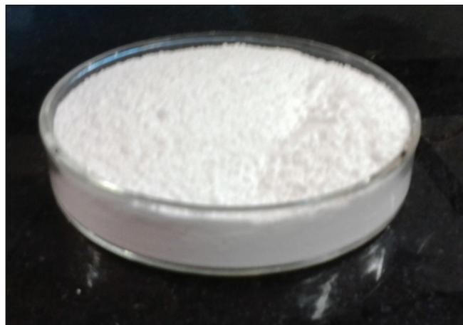
Fig. 1: Silver-doped hydroxyapatite in powder form
