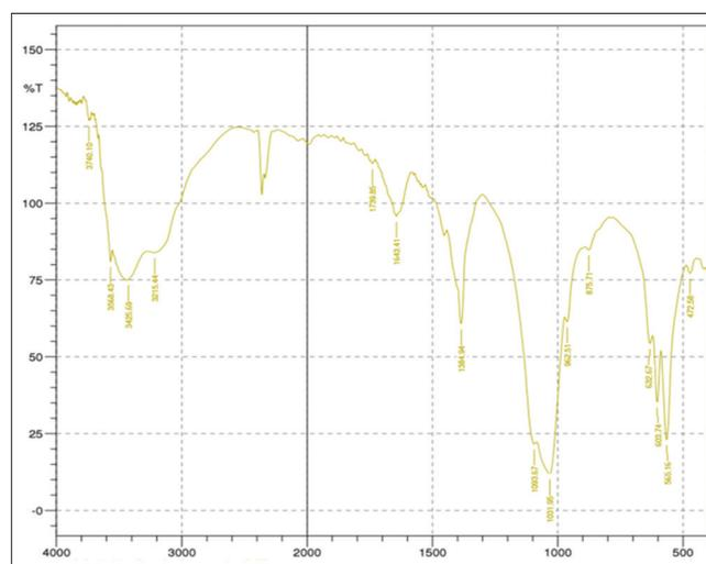
Fig. 3: Fourier transform infrared spectroscopy spectra from silver-doped hydroxyapatite
