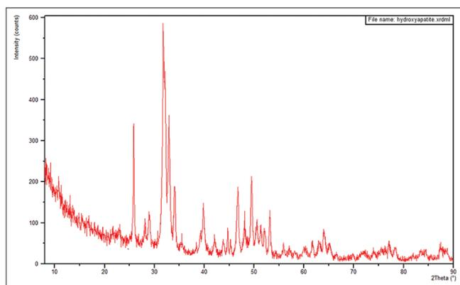
Fig. 4: X-ray diffraction spectra of synthesized silver-doped hydroxyapatite
