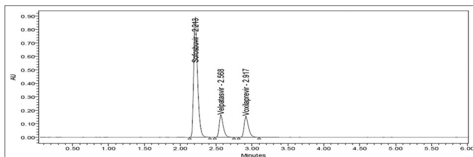
Fig. 4: Typical optimized chromatogram of sofosbuvir, velpatasvir, and voxilaprevir
