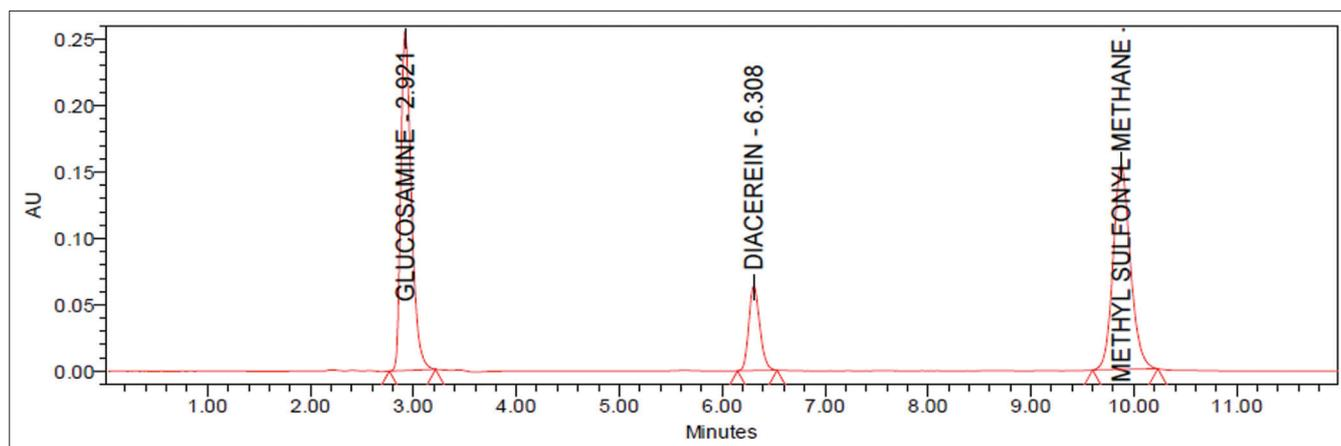
Fig. 7: Chromatogram for system suitability
