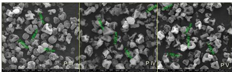
**Fig. 1: Scanning electron microscope of ketoprofen-carboxymethyl chitosan dried at different condition: 100°C, pump rate 3.5 ml.minutes (P III), 9 ml/minutes (P IV); 120°C, 3.5 ml/minutes (P V) (magnification ×10,000)**
