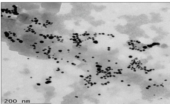
Fig. 5: High-resolution transmission electron spectroscopic image of AgNPs (scale bar 200 nm)
