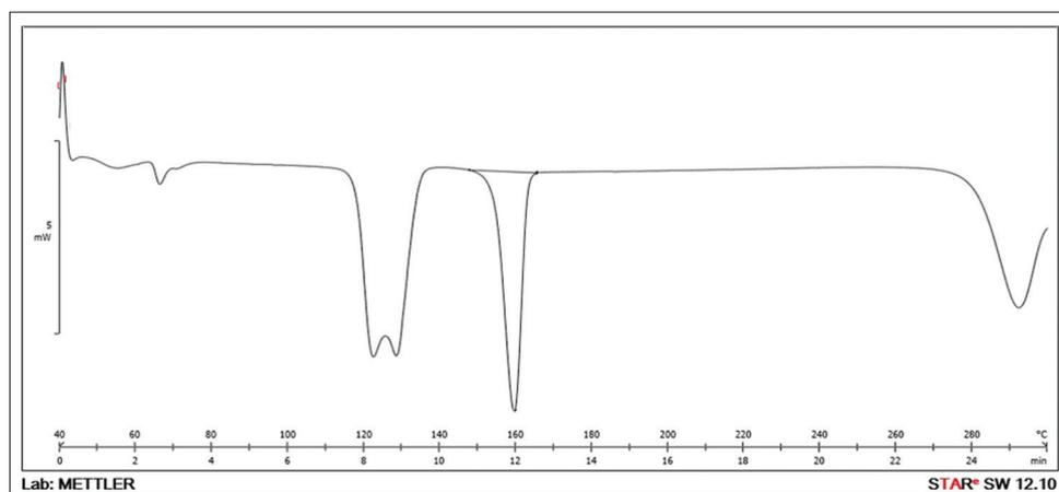
Fig. 2: Differential scanning calorimetry of apremilast cocrystals
