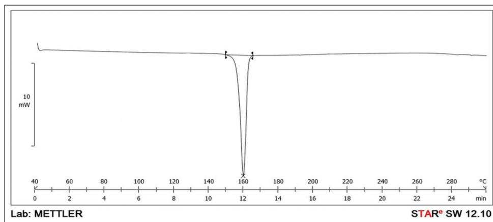
Fig. 1: Differential scanning calorimetry of pure apremilast
