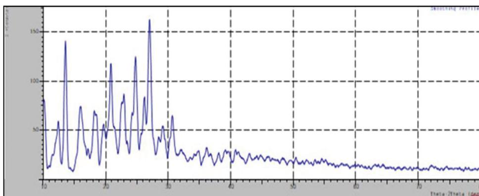
Fig. 4: X-ray diffraction of apremilast cocrystals
