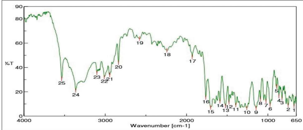
Fig. 6: Fourier-transform infrared spectra of apremilast cocrystal
