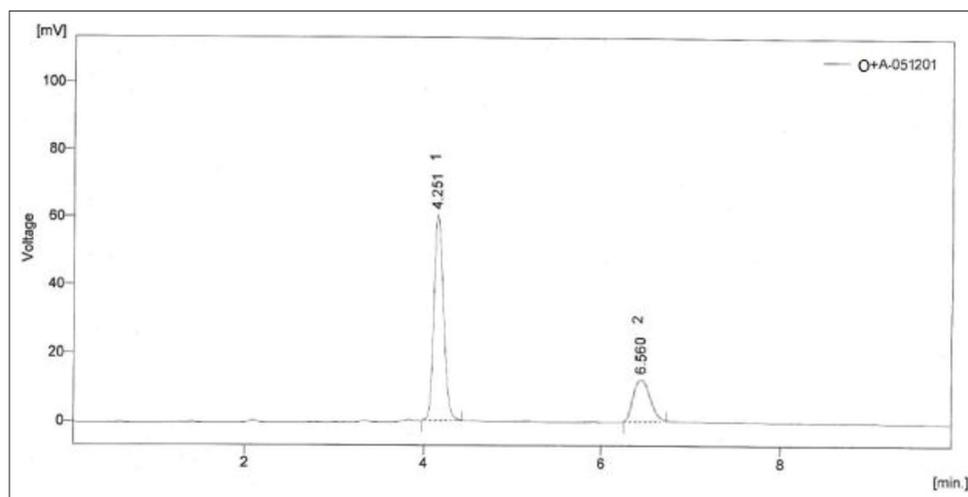
Fig. 9: Chromatogram of binary mixtures (olanzapine + aripiprazole)
