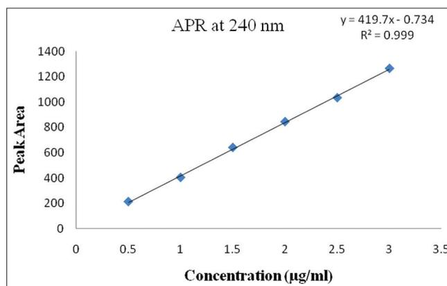
**Fig. 6: Calibration curve of aripiprazole (0.5–3.0 µg/ml)**
