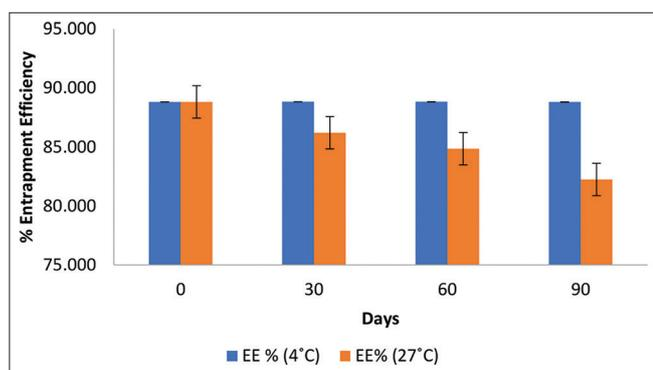
Fig. 6: Effect of storage temperature (at 4°C and 27°C) on Entrapment Efficiency of F10
