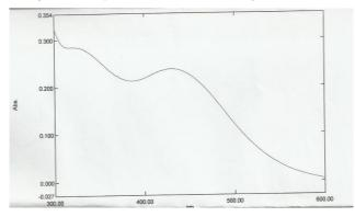
Figure2a : UV-VIS spectrum of Ag nanoparticles under optimum conditions
