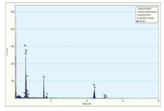
Figure 9: EDAX spectra of Silver Nanoparticles
