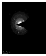
Figure 8c: Selected area Electron Diffraction Pattern (SAED)
