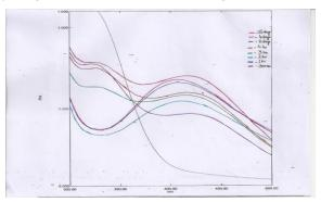
Figure 4: UV- VIS spectra of Silver Nanoparticles showing stability
