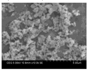
Figure 7: SEM micrograph of Silver Nanoparticles.
