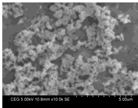
**Figure 7: SEM micrograph of Silver Nanoparticles.**
