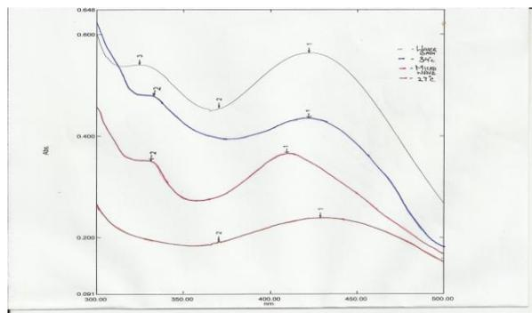
Figure 2b: UV-VIS absorption of Ag Nanoparticles synthesized at different and under different heating conditions
