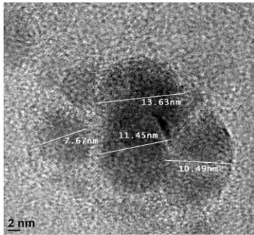
Figure 8b: Nanoparticles showing capping
