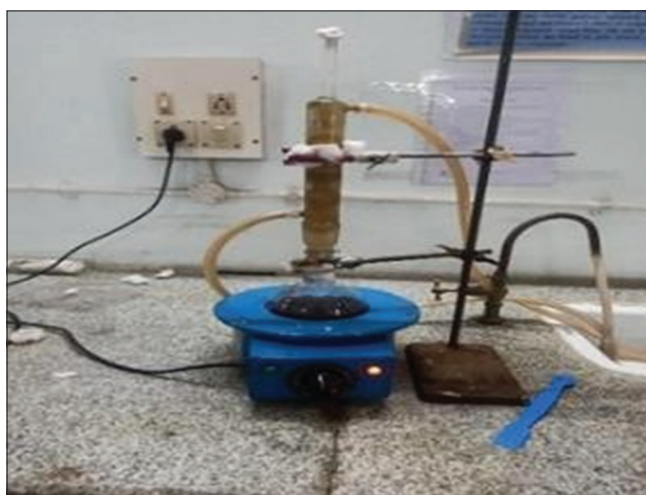
Fig. 2: Extraction performs using the decoction method
