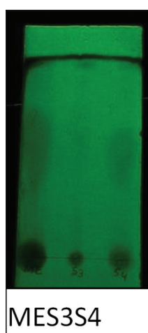
Fig. 11: Thin-layer chromatography of ethanolic extract of Agaricus bisporus with the respect of chloroform and n-hexane
