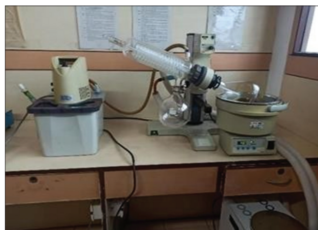
Fig. 3: Ethanol evaporation using rotary evaporator
