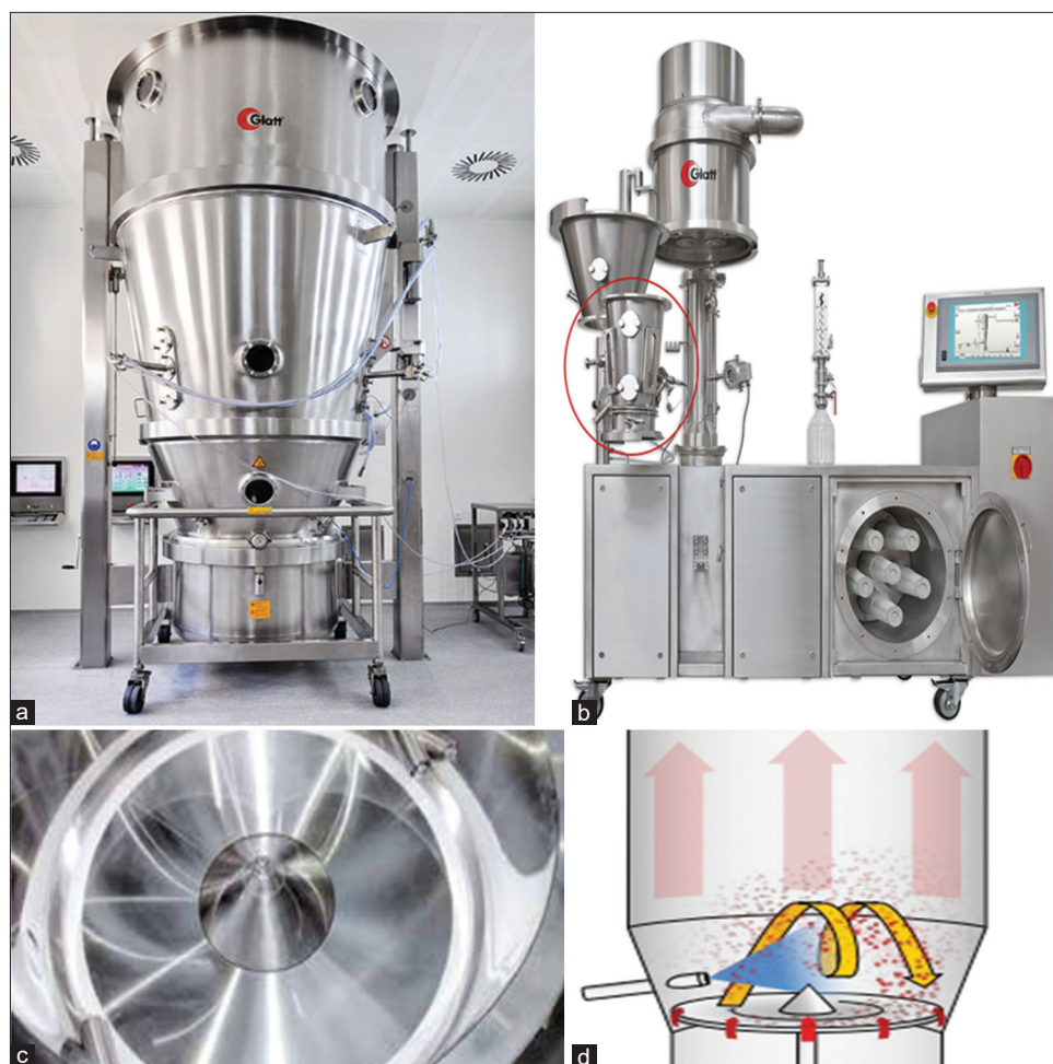
Fig. 6: (a) Fluid bed granulator and coater GPCG 300 at the glatt technology center in Weimar, Germany (b). Mobile glatt fluid bed/spouted bed laboratory unit ProCell® LabSystem at the glatt technology center in Weimar, Germany, with six modular all-rounder system (c and d). Tangential spray in rotor insert (Glatt)
