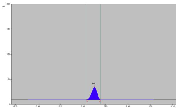
Fig. 1: Densitogram of BHT ( $R_f$  0.49), detection at 254 nm
