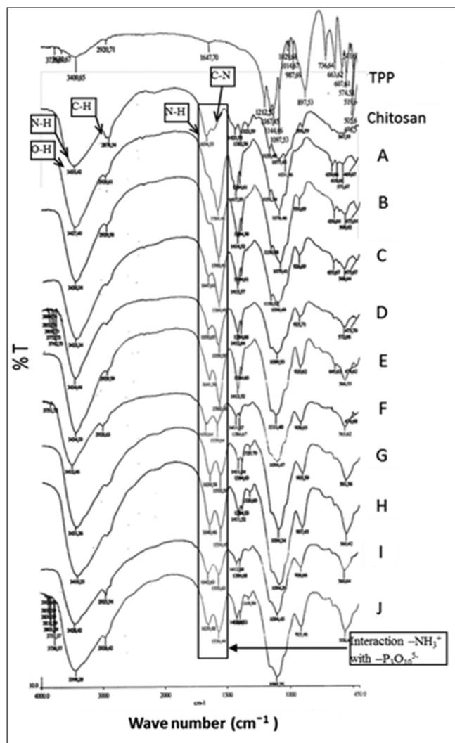
**Fig. 1: Fourier transform infrared spectra of tripolyphosphate (TPP), chitosan and unloaded chitosan particles with chitosan-TPP ratio: 10:1 (A), 10:2 (B), 10:3 (C), 10:4 (D), 10:5 (E), 10:6 (F), 10:7 (G), 10:8 (H), 10:9 (I), 10:10 (J)**
