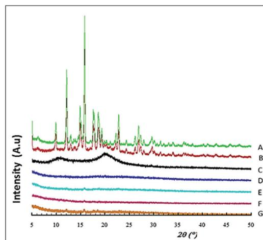
Fig. 6: X-ray diffractogram of the diterpene lactone fraction of sambiloto (FDTL) (A), physical mixture FDTL-chitosan (B), chitosan (C), unloaded particles (D), FDTL loaded particles with FDTL-chitosan-tripolyphosphate ratio 3:10:8 (E), 4:10:8 (F), 5:10:8 (G)
