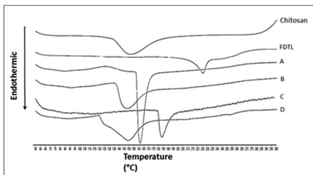
Fig. 5: Differential thermal analyzer thermogram of chitosan, diterpene lactone fraction of sambiloto (FDTL), and unloaded particles (A), FDTL loaded particles with FDTL-chitosan-tripolyphosphate ratio 3:10:8 (B), 4:10:8 (C), 5:10:8 (D)
