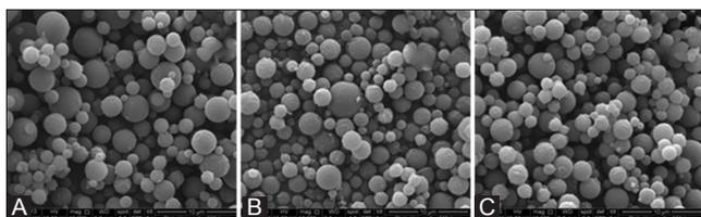
Fig. 3: Scanning electron microscope photograph of diterpene lactone fraction of sambiloto (FDTL) loaded chitosan particles with FDTL-chitosan- tripolyphosphate ratio: 3:10:8 (A), 4:10:8 (B), 5:10:8 (C) (magnification,  $\times 10,000$ )
