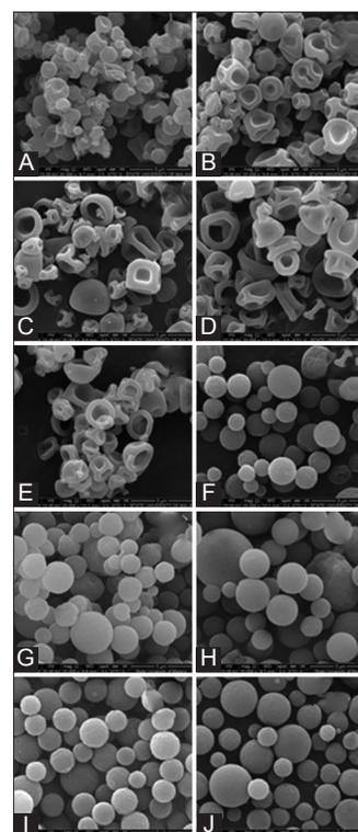
**Fig. 2: Scanning electron microscope photograph of unloaded chitosan particles with chitosan-tripolyphosphate ratio: 10:1 (A), 10:2 (B), 10:3 (C), 10:4 (D), 10:5 (E), 10:6 (F), 10:7 (G), 10:8 (H), 10:9 (I), 10:10 (J) (magnification,  $\times 20,000$ )**
